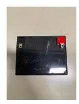
4. Install the new battery by reversing the steps above, connecting both the black and red wires onto the new battery. Be careful to connect the red wire to the red battery tab and the black wire to the black battery tab. If you reverse the wires, you will ultimately melt your battery which could result in a fire.
